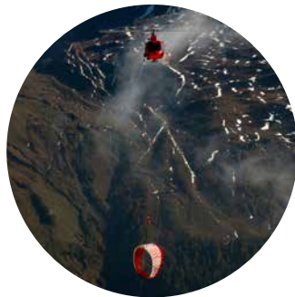
Step 2 The final transport of each unit is made by ordinary grade helicopters (B3).
